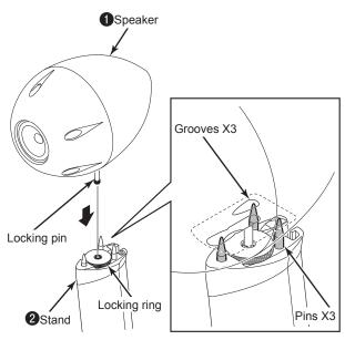
Tighten the locking ring to secure the speaker to the stand.
