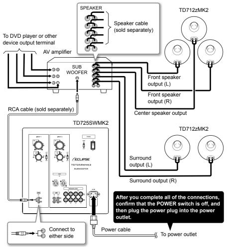
If your AV amplifier has only one subwoofer output channel, connect the cable to either line-in terminal, or use a splitter cable (sold separately) and connect the cables to both line-in terminals.
