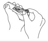
3 Push the rear cover in the direction of the arrow to close the battery case.
