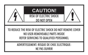
This lightning flash with arrowhead symbol within an equilateral triangle is intended to alert the user to the presence of non-insulated "dangerous voltage" within the product's enclosure that may be of sufficient magnitude to constitute a risk of electric shock.
