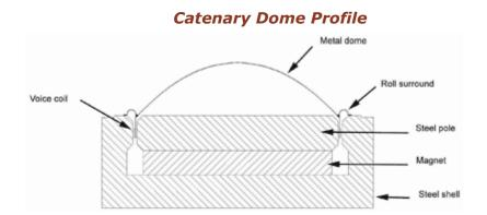
At Vivid Audio we believe in using pistonic drivers for every part of the spectrum because we have found, though experience and experiment, that no matter how well controlled it may be, cone break-up is always audible as a colouration of the sound. There may well be times when that colouration produces a pleasant effect but we feel that effects should be included by the artist in the recording and not be added later during the reproduction.
