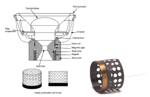
In a manner reminiscent of a piston in a cylinder, the central pole of the magnet in a standard moving coil driver alternately compresses and rarefies the air trapped within the voice coil, behind the dust dome. There is an escape route through the narrow gap between the coil and pole but the air experiences considerable drag which in turn damps the motion of the cone, particularly at low frequencies where the displacement is greatest.
