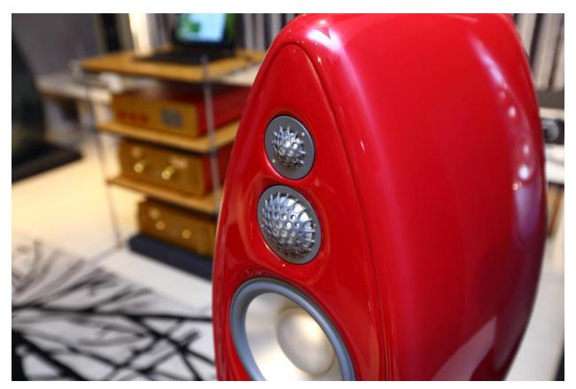
In Vivid Audio design, woofer design is the most special, B1d front and back of the woofer is the same, Vivid Audio uses two identical woofers in the opposite direction, is to offset the woofer movement the reaction force generated when, Philip Guttentag think the best way is the reaction slashing motion across monomer to give him one and the same force, rather than the quality of housing in most of the large rigid suppression.
