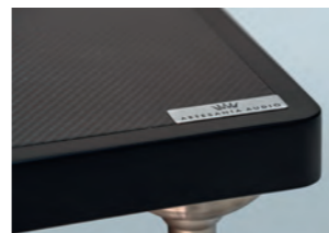
CARBON FIBER / GLASS FIBER / KRION / MDF MULTILAYER PLATFORM Carbon fiber 100% 3K Twill 200gr/m2 on both upper and lower faces, with G10 biaxial glas fiber 180 gm/m² inner core. Finishing like fiber arms.
