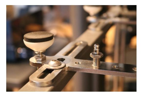
Above: if so desired, the M8 bolts could also be used to replace the standard Artesania level footers, although I would not recommend this as the footers may damage components stacked below if they slip away.
