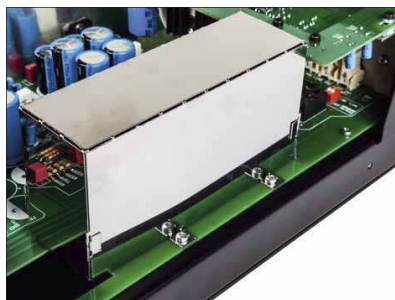
The delicate signal from the cartridge is treated under the cover of a metal shield.
