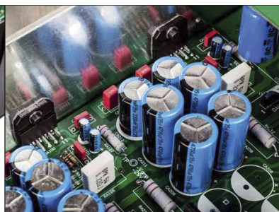
The output stage of the 404 uses tried and tested amps on a chip/power amp components
