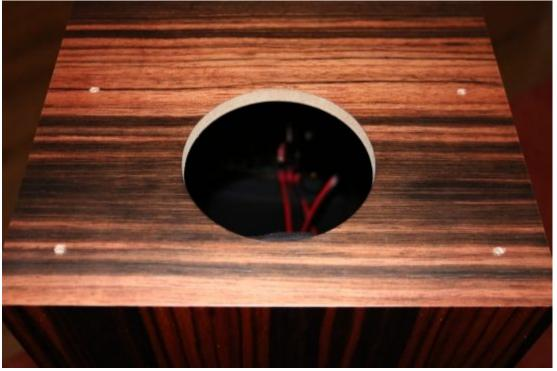
Above and below: the bass reflex holes are directly open to the speaker's internal air mass, they do not have a tube.
