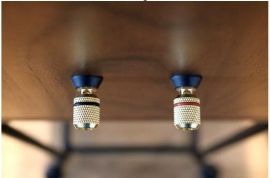
The notched connectors offer only a very small contact area when using Spades. It works well enough, but for a better and more reliable connection with a wide range of spades, I had preferred a larger flat surface area. The manufacturer commented that they use bananas exclusively.
