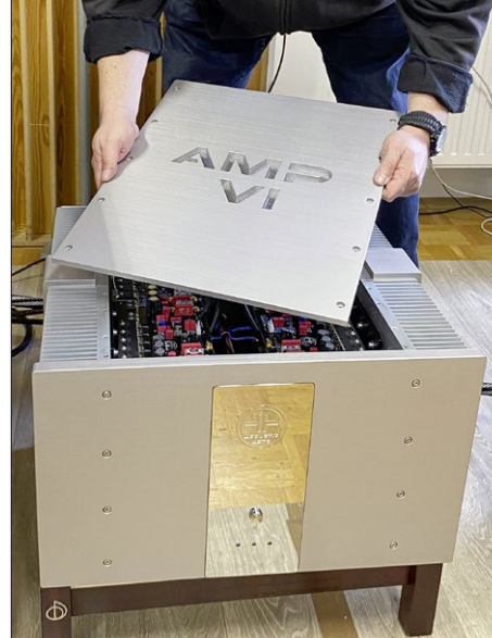
The cover plate alone, milled from solid brass, is basically as thick as a finger.
