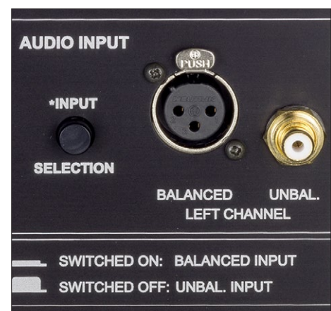
The similarly high-quality RCA and XLR input sockets are switchable.
